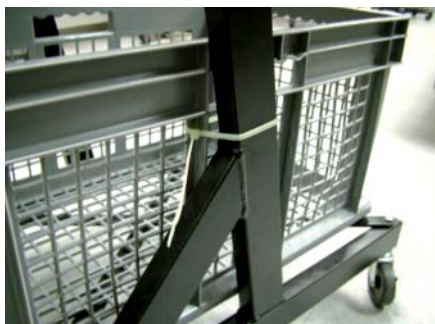
Attach Longer Cable Tie to Side Post
