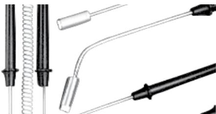
Choose these probes for economy. Each probe has a 304 stainless steel sheath. 3-foot, color-coded PVC cable and color-coded mini-connector. Integral Handle Probes have a 20 gauge coiled cable. Each probe has a characteristic time constant (response time). Five time constants are needed to reach 99% of final reading.
